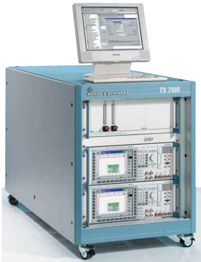
TS7100: example of a 2-channel ultra- low-profile config- uration with PSU and switch matrix fitted to rear of rack
