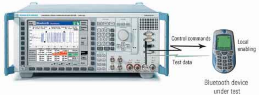
The device under test can be connected to the CMU200 via an RF coupler (antenna) or a cable
